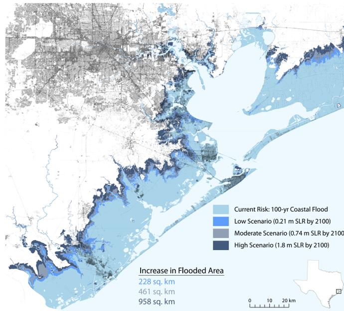
**Figure 3:** Extent of inundation due to a 100-year coastal flood with present-day sea level (Current Risk) and due to 3 SLR scenarios in 2100 on top of 100-year flood.
